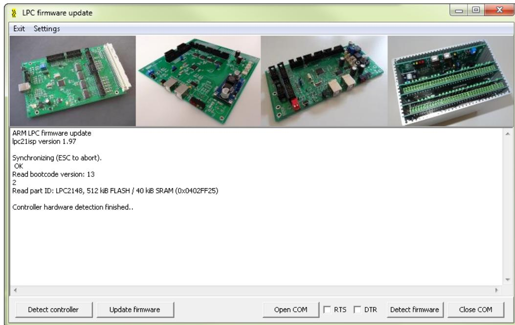
If the USB-RS232 firmware has been installed, a firmware detection can be performed. Open Com port, reset the controller using DTR/RTS or do it manually and then press “Detect firmware”.
