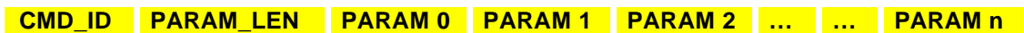
Figure 1 : Structure of a command that will be understood by the AKKON USB CNC controller kernel
